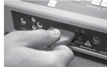
Figure 3. Plug the 3-prong power cord into the electro-surgical generator of your choice, (Figure 3). Confirm that all power settings on the generator are appropriate for the procedure being performed. The electrosurgical generator's intensity should be set as low as is necessary to achieve the desired effect. The PlumePen® Elite is a monopolar electrode, the use of a dispersive electrode is required to prevent burns/injury to patient. Please refer to electrosurgical generator user manual and dispersive electrode instructions for use for additional instructions.
