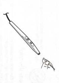
Ensure the insulating sleeve fits securely inside the nose of the pencil so that the nose overlaps the insulating sleeve by at least 1/8" (0.3 cm).
