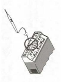
Grasp the insulating sleeve on the electrode, and insert the electrode into the pencil.
