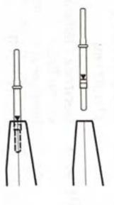
A tip protector covers the coated end of some electrodes. If a tip protector is present, remove it before use.
