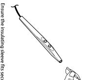
Ensure the insulating sleeve fits securely inside the nose of the pencil so that the nose overlaps the insulating sleeve by at least 1/8" (0.3 cm).
